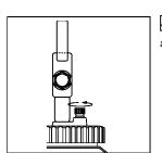
Job 1 When you interrupt a job or replenish paint, be sure to turn off air supply to spray gun and pressurized container, open release valve and release pressure in pressurized container.
