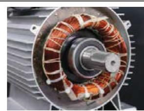
Copper wound motors provide longer lasting performance over aluminium wound motors.
